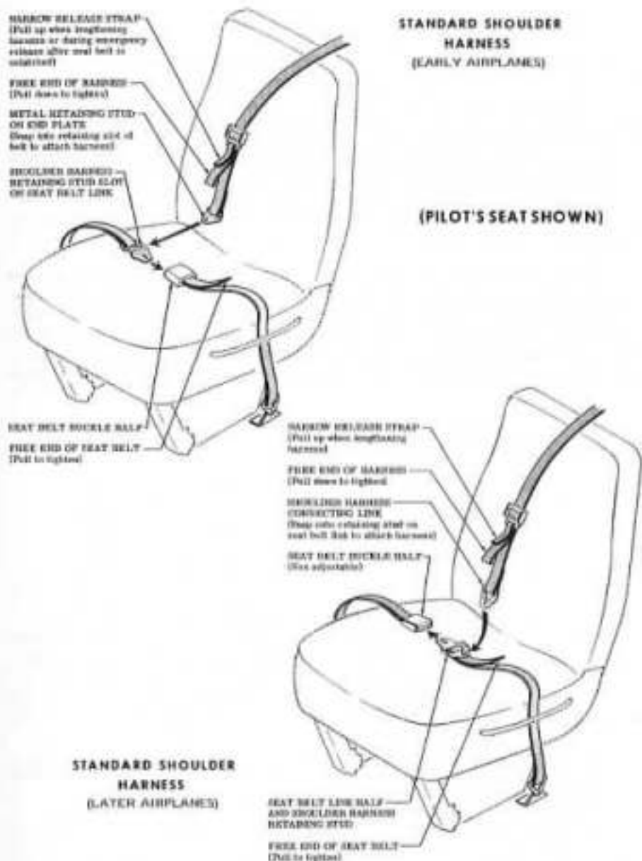
Figure 7-4. Seat Belts and Shoulder Harnesses (Sheet 1 of 2)
